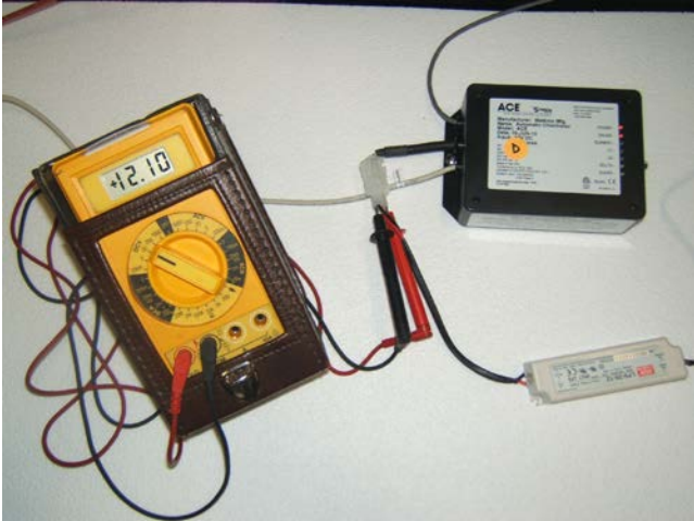
a) 11.5VDC minimum from the power supply to the controller.
