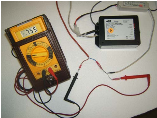
c) 500 mA DC – 1200 mA DC at the cell. (Element LED on the controller must be ON)
